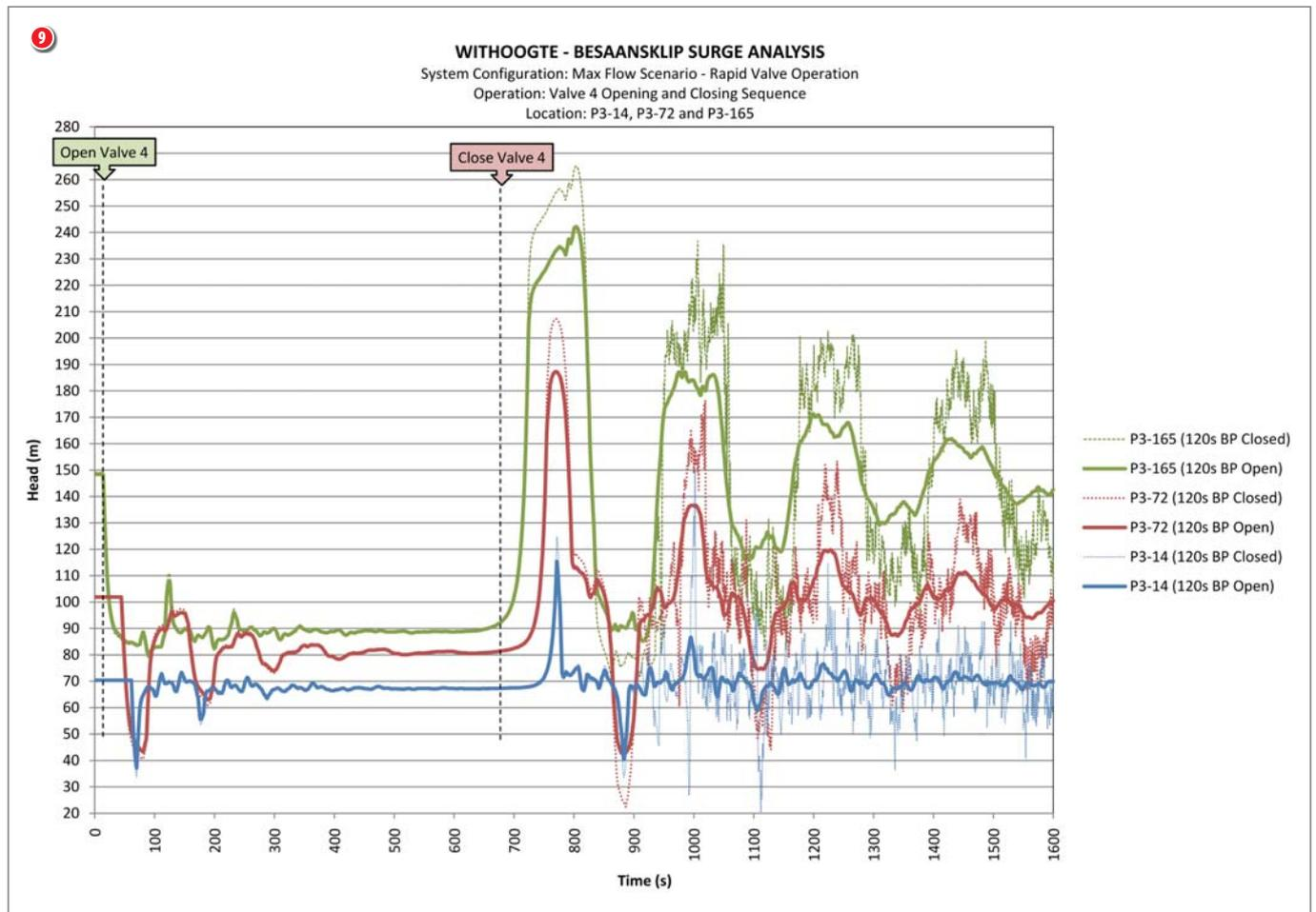
celerity and transient behaviour of the system were therefore accurately reflected by the Surge 2010 hydraulic model, and the model could be used with confidence to analyse further operational scenarios. Figures 4 and 5 illustrate the correlation between the measured and modelled pressure variation following the execution of similar operational changes in the physical and simulated environments.
