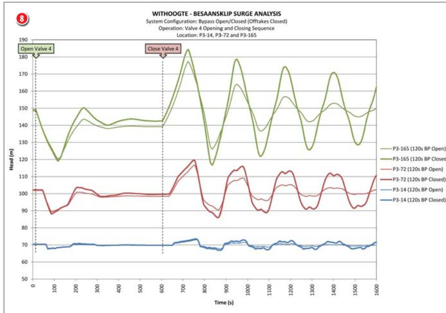
8 Modelled pressure variation at different locations along the pipeline with the by-pass on the Besaansklip inlet manifold open and closed
