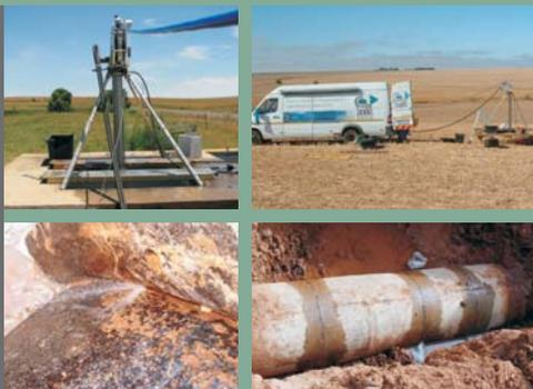
Acoustic leak detection and CCTV inspections are performed in real time, under pressure and uninterrupted, without the need for costly, high risk, pipeline shut-downs.
