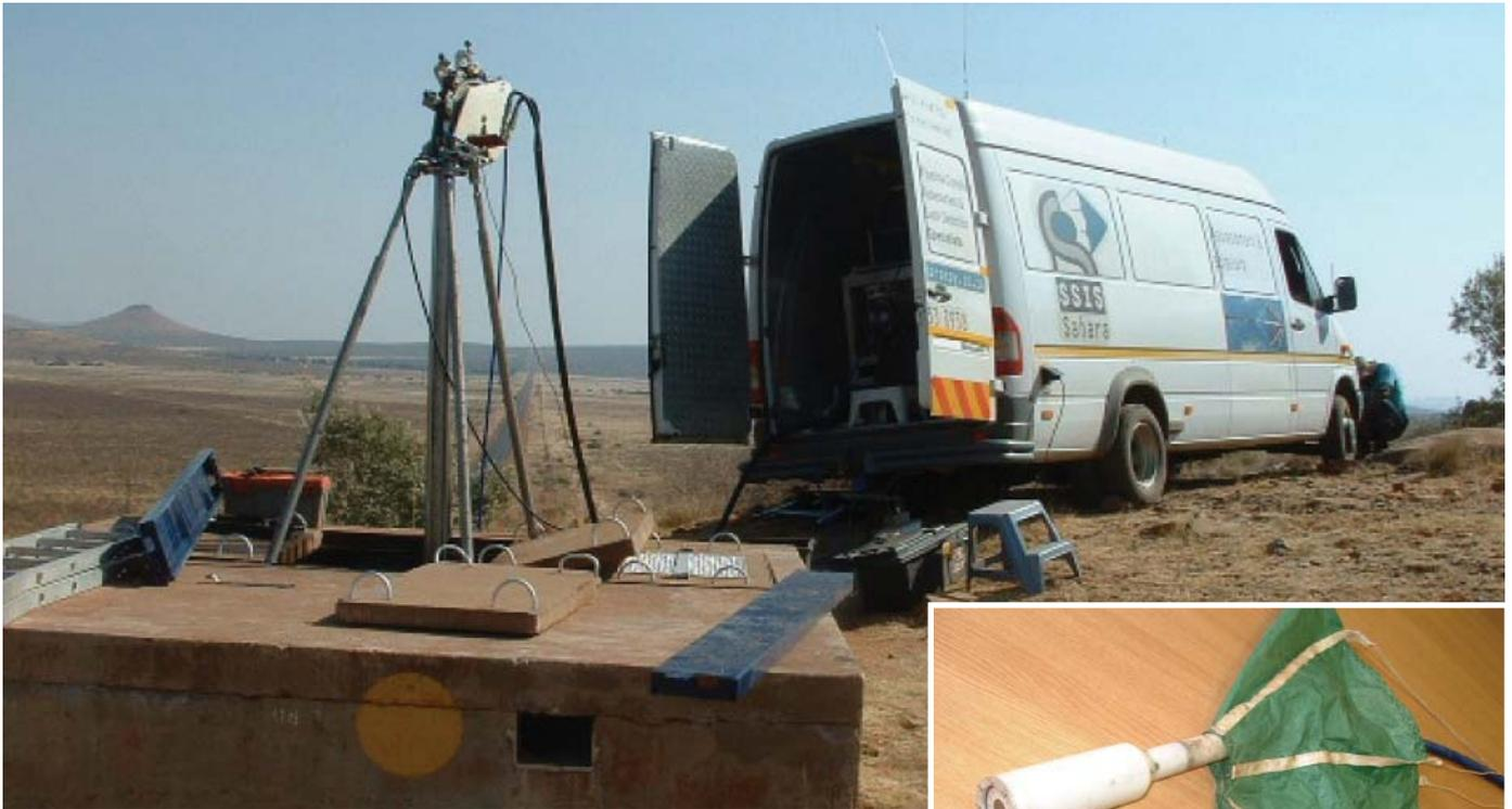
head, inspection cable and parachute are then deployed under pressure through the insertion tube into the pipeline while the pipeline remains in service. The flow of water opens the parachute and provides the necessary drag to pull the camera and cable along the pipeline (refer to figures 2 and 3).
